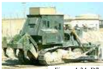
Figure 4-34: D7 Dozer with MCAP
