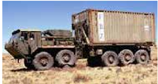
Figure 1-47: LVSR-18 with Steel 20-foot Sea Container
